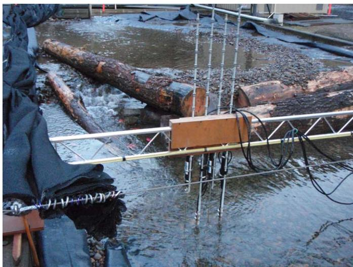
**Figure 1.** Experimental channel and ADV setup. Image is oriented looking upstream.
